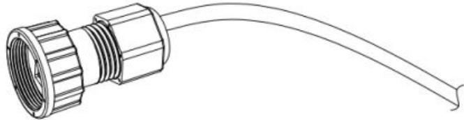
Step 2: Crimp the cable with a RJ45 plug which is inside of the cable connector.
